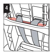
Pull harness through the back. Make sure the harness goes OVER the metal bar, BETWEEN metal bar and plastic handle of the harness/headrest adjuster.
